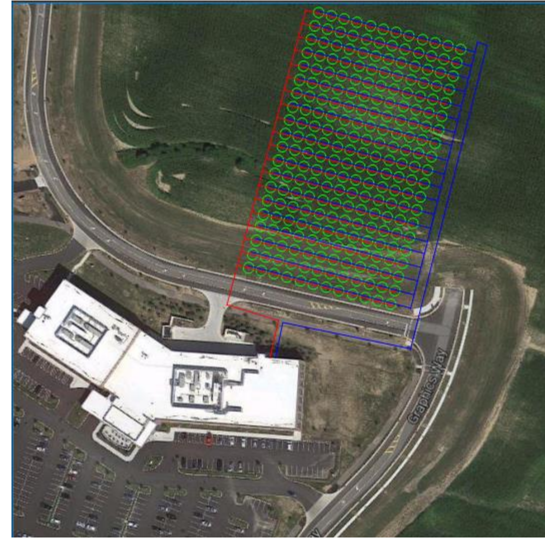
Geothermal Well Field Layout
